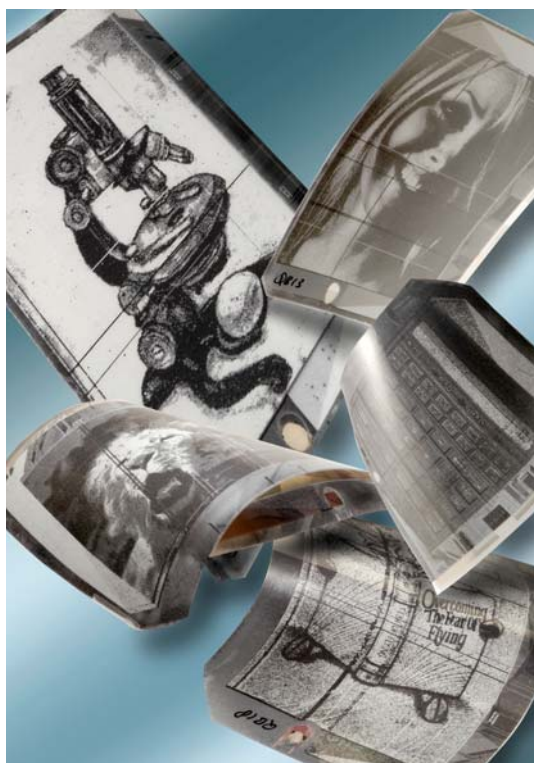
Figure 56. Flexible active-matrix displays using Philips' ultra-thin back plane with organics-based thin film transistors, combined with E Ink's electronic ink front plane. Photo: Philips.
