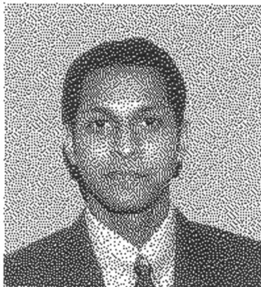
Figure 50. A visually-significant barcode, developed by HP Labs. Copyright (2007) Hewlett-Packard Development Company, L.P. Reproduced with permission.
