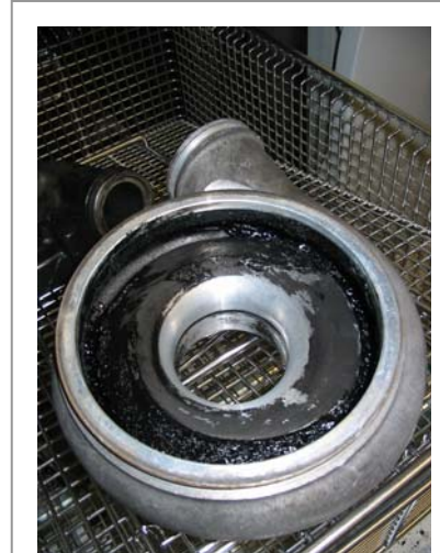
Design for Reconditioning may reduce the use of forms that gather dirt
